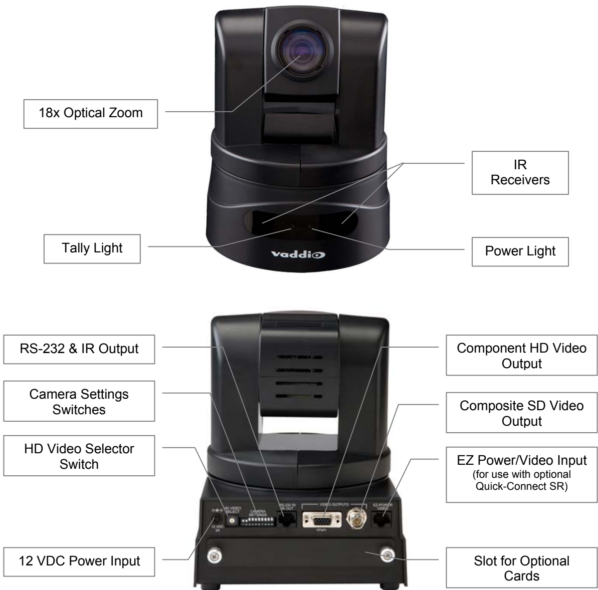
Figure 2: ClearVIEW HD-18 front and rear diagrams with functional callouts.
